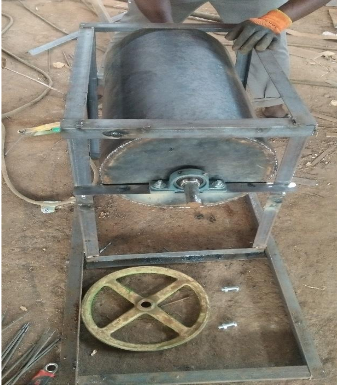
FIGURE 6: ASSEMBLING OF THE SHELLING CHAMBER
